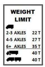
To ensure uniformity in all postings, the above signs are to be used for the various types of bridge load postings.
